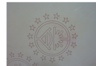
Marking color change coating 1,4 W CO 2 laser, 18 m/min
